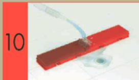
Rinse pads using moderate water pressure.
