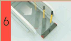
Place the device onto the moving treads, allow it to align with the combs and drop into place.
